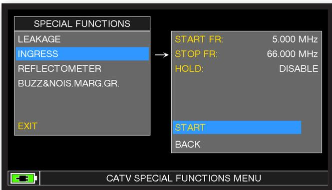
Set the desired parameters, at the end touch "START" to start the Ingress measures.
