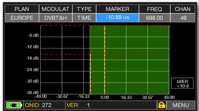
MicroEchoes visualization, touch the Marker and rotate the encoder to select the ECHOES.
