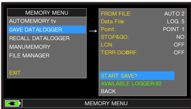
Touch "SAVE DATALOGGER" and set the parameters required. Touch "START SAVE" to create a new log file.
