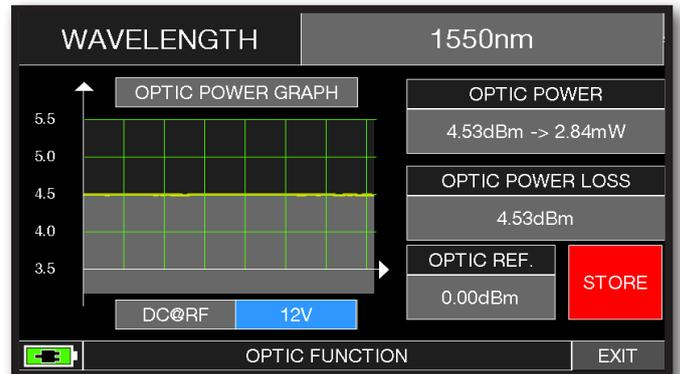
Touch "DC@RF" and, if required, select the power supply voltage: for Example 12V.
