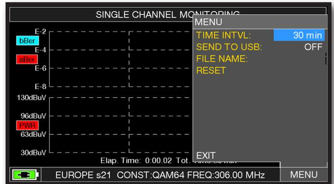
Select the time interval (TIME INTVL) and where you want to store the file, either in the meter's memory, or in the USB memory stick (send to USB-ON), with the relative file name (File name).
