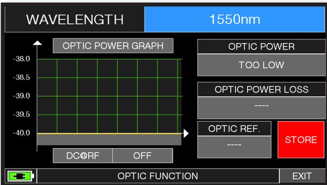
Touch "WAVELENGTH" and select the Wave length desired: for Example 1550 nm.
