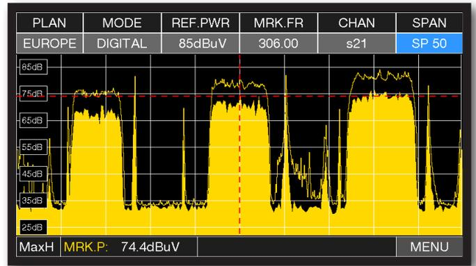
Press again to spectrum key to activate the "MAX HOLD" function.
