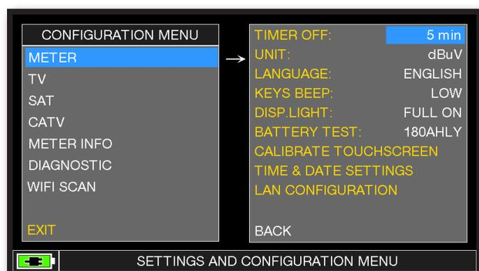
Touch "CONFIGURATION MENU" then "METER" in the volume screen and set the "TIMER OFF" value required. The meter will turn off after 5, 10, 15 or 30 minutes of inactivity. Press any key to interrupt the automatic turn-off.
