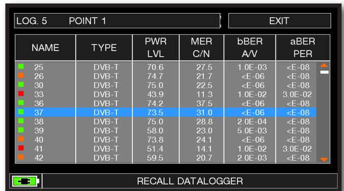
Example of saved measured in the Log file. Touch the screen to browse through measurements saved in the log file.
