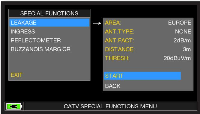
Set the desired parameters, at the end touch "START" to start the leakage measures.
