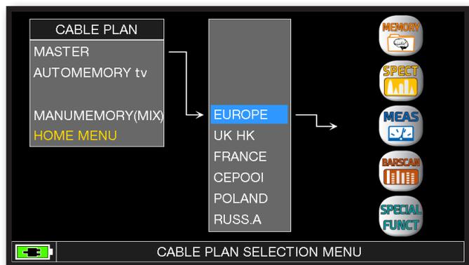
Touch directly the decided canalization or use the encoder. At the end touch "MEAS" to make the measure or "SPECT" for visualize the spectrum.
