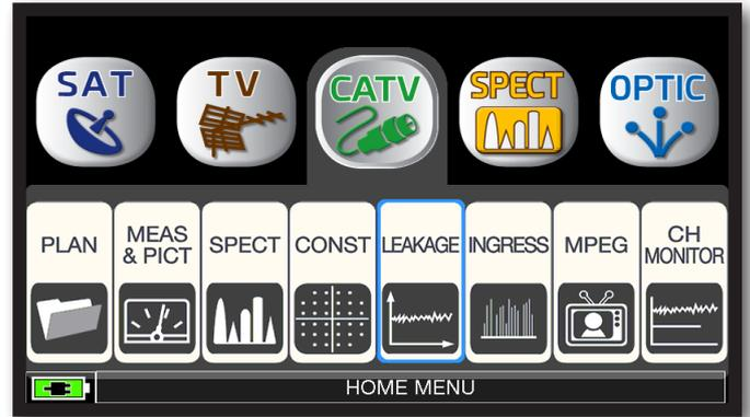
Touch "CATV" and then "LEAKAGE" or use the encoder.
