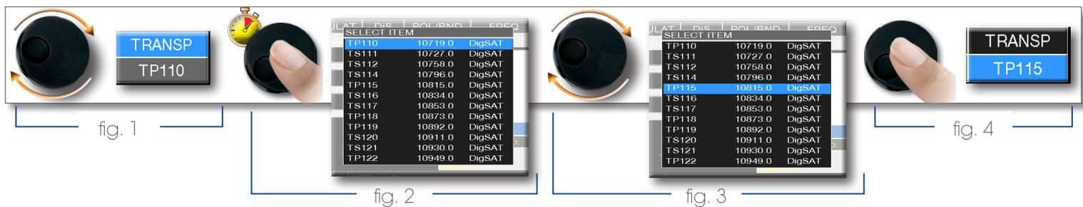
How to select the frequency and set the value using the numerical keyboard:
