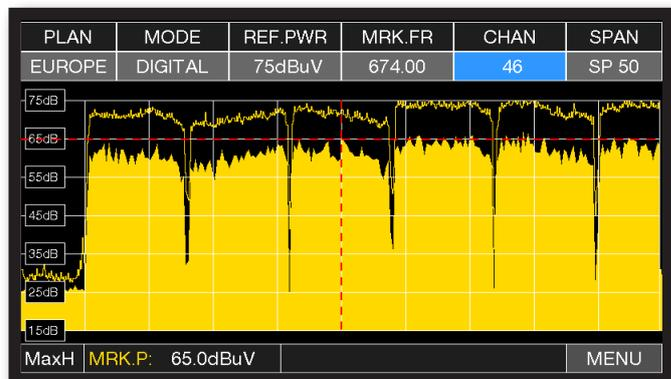
Press again to spectrum key to activate the "MAX HOLD" function.
