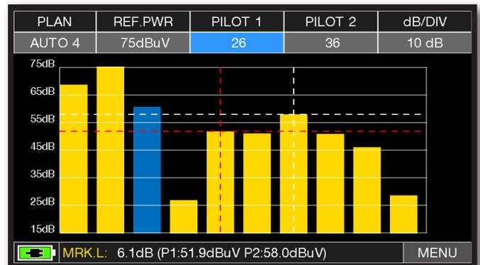
BARSCAN (TILT GRAPHIC). Touch "PILOT 1" and "PILOT 2" to select the two channels to be used for the tilt measurement (level difference).
