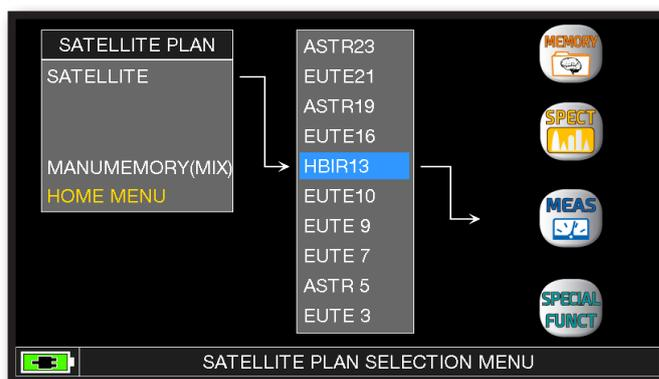
Touch directly the desired satellite, or use the encoder. At the end touch "MEAS" to make the measure or "SPECT" for visualize the spectrum.
