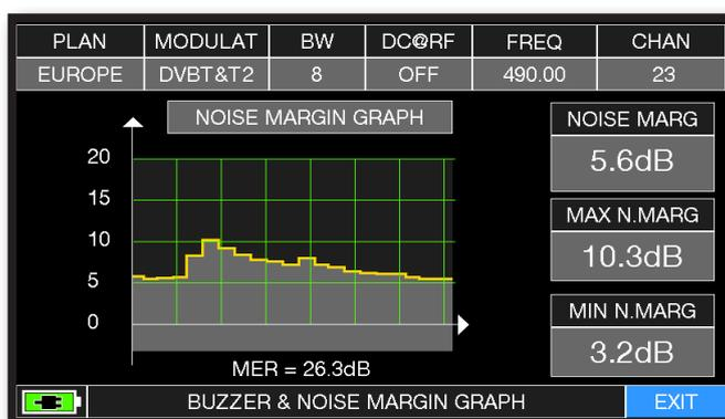
Buzzer & Graphic of the progress of the noise NOISE MARGIN of the TV/CATV tuned channel according to time.
