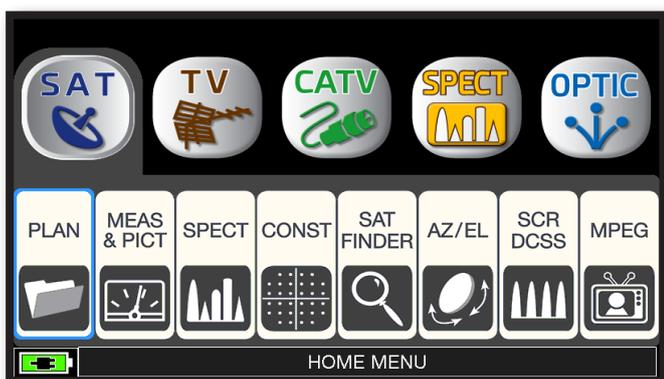
Touch "SAT", and then "PLAN" or use the encoder to obtain the Satellite list.
