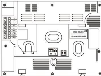
Remove the bracket installation of the monitor.
