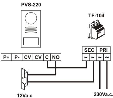
Use an external relay for devices with higher consumption than 12Vd.c. / 1A.
