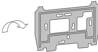
**F**ix the bracket installation to the wall.
