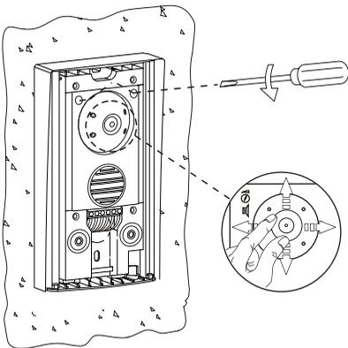
If after starting the system it's considered that the audio volume isn't correct, proceed with the necessary adjustments as shown on the picture.
