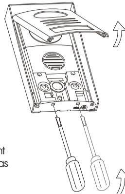
With help of a plain screwdriver, remove the aluminium front making a light pressure in the door panel bottom holes, as shown on the picture.
