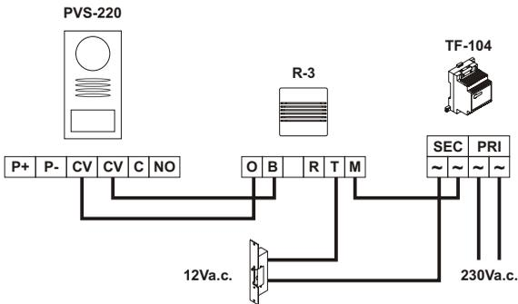
Connection of an auxiliary device.
