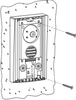
Face the door panel to the wall by placing the top at 1,65m. height and insert the installation wires through the cables entry.
