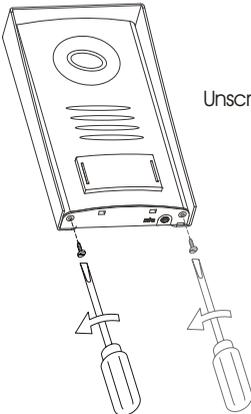
Unscrew the door panel bottom screws.
