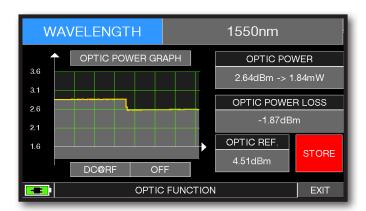
In the "OPTIC POWER LOSS" field, the optical attenuation value is displayed with respect to the stored value (Optic REF):
