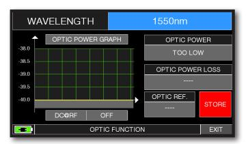
Touch "WAVELENGHT" and select the Wave length desired: for Example 1550 nm.
