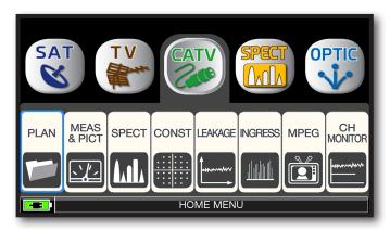
Touch "CATV" and then "PLAN" or use the encoder to access at the CATV canalizations list.
