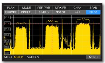
Press again te spectrum key to activate the "MAX HOLD" function.
