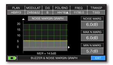
Buzzer & Graphic of the progress of the NOISE MARGIN of the tuned Sat Transponder according to time.
