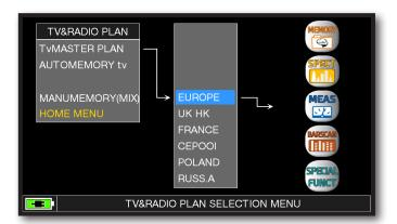
Touch directly the desided canalization or use the encoder. At the end touch "MEAS" to make the measure or "SPECT" for visualize the spectrum.
