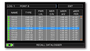
Example of saved measured in the Log file. Touch the screen to browse through measurements.
