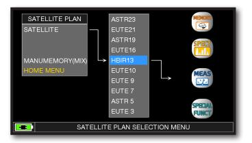
Touch directly the desided satellite, or use the encoder. At the end touch "MEAS" to make the measure or "SPECT" for visualize the spectrum.
