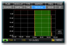
Fig. 3: MARGINAL RECEPTION (or IMPOSSIBLE):\* 2 ECHOES present outside the guard interval mask (green area), coming from a distance of: 1st echo:
