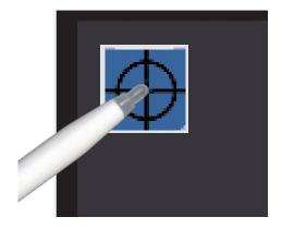
**NOTE**: use the pen and touch the the screen exactly in the center of the circle. if you do not carry out this procedure correctly the touch commands may be inaccurate.
