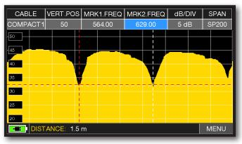
In the DISTANCE window, read the cable's mismatching value: example 1.5 m.
