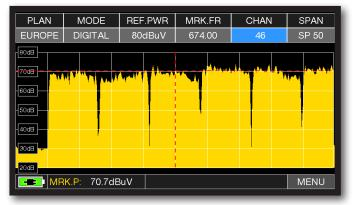
TV spectrum SPAN 50 MHz
