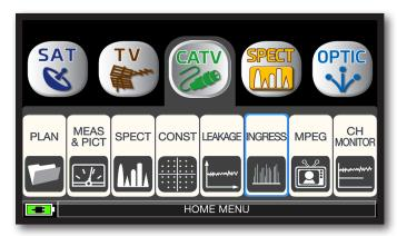
Touch "CATV" and then "LEAKAGE" or use the encoder.
