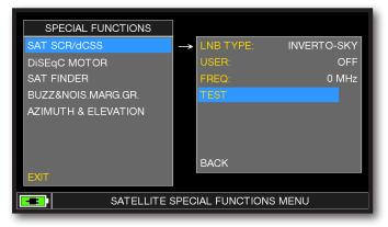
Or touch "TEST", in Spectrum mode, to perform a verify of the 8 exit frequencies (user 1-4) from LNB/multiswitch.
