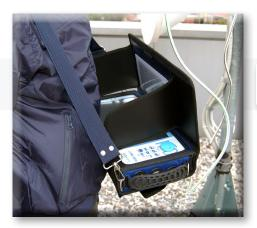
The sunlight shield flap allows improved visibility of the high brightness display.
