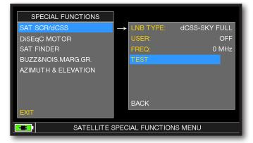
Or touch "TEST", in Spectrum mode, to perform a verify of the 8 exit frequencies (user 5-16) from LNB/multiswitch.
