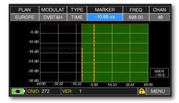
MicroEchoes visualization, touch the Marker and rotate the encoder to select the ECHOES.
