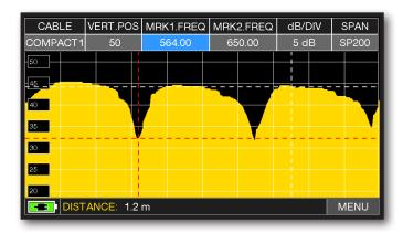
Touch "MRK1.freq" then "MRK2.freq" and set the marker frequencies in correspondence with the first and second minimum points.
