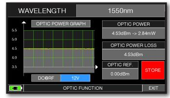
Touch "DC@RF" and, if required, select the power supply voltage: for Example 12V.
