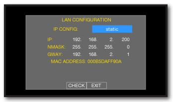
Touch "IP CONFIG" and select "STATIC", insert the "IP", "NMASK" and "GWAY" parameters.
