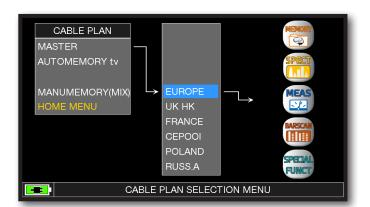
Touch directly the desided canalization or use the encoder. At the end touch "MEAS" to make the measure or "SPECT" for visualize the spectrum.
