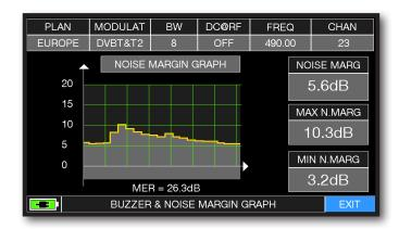
Buzzer & Graphic of the progress of the noise
