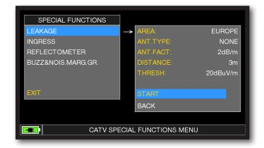
Set the desired parameters, at the end touch "START" to start the leakage measures.
