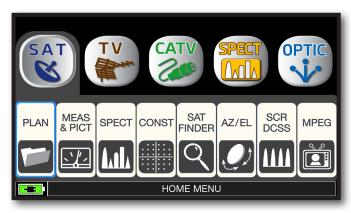
Touch "SAT", and then "PLAN" or use the encoder to obtain the Satellite list.
