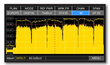
Press again te spectrum key to activate the "MAX HOI D" function.
