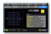
The table to the right shows all the received modulation parameters
