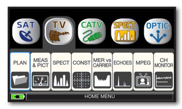
Touch "TV" and then "PLAN" or use the encoder to access at the TV canalizations list.
