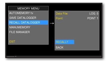
Touch "RECALL DATALOGGER" and Set the LOG file parameters.
