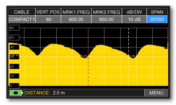
Touch "SPAN" and select the correct visualization value.
